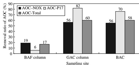
Fig. 5. AOC removal efficiency of the column test.
