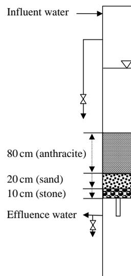
Fig. 2. The diagram showing the components of the glass column.
