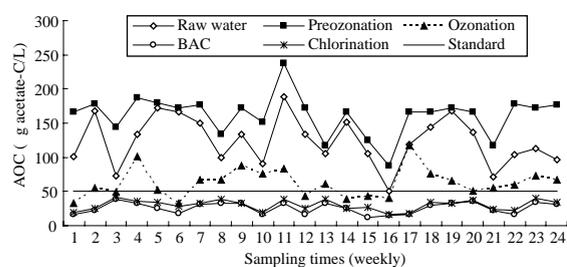
Fig. 3. AOC concentrations in the effluent of various treatment processes.
