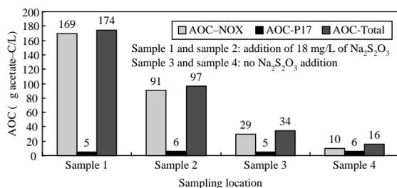
Fig. 4. Effect of sodium thiosulfate addition on AOC measurement (samples 1 and 3: effluences of preozonation, samples 2 and 4: effluences from chlorination).
