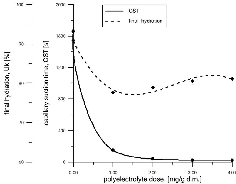
Fig.2. The influence of polyelectrolyte Zetag 92 dose on sludges dewatering parameters
