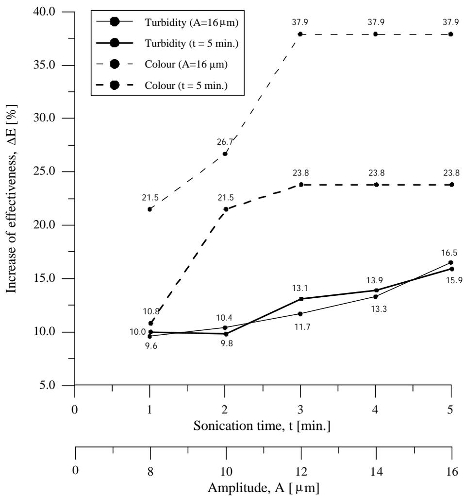
Fig.1. Dependence of the increase of effectiveness in water turbidity and colour reduction on the vibration amplitude and sonication time in the US+C system
