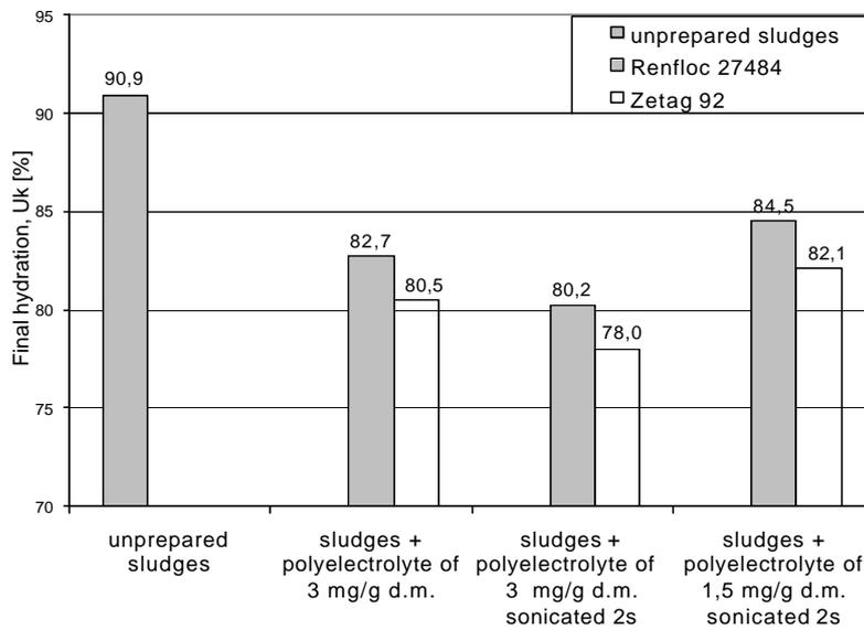
Fig.3. Changes of sludges final hydration conditioned with polyelectrolytes before and after sonification
